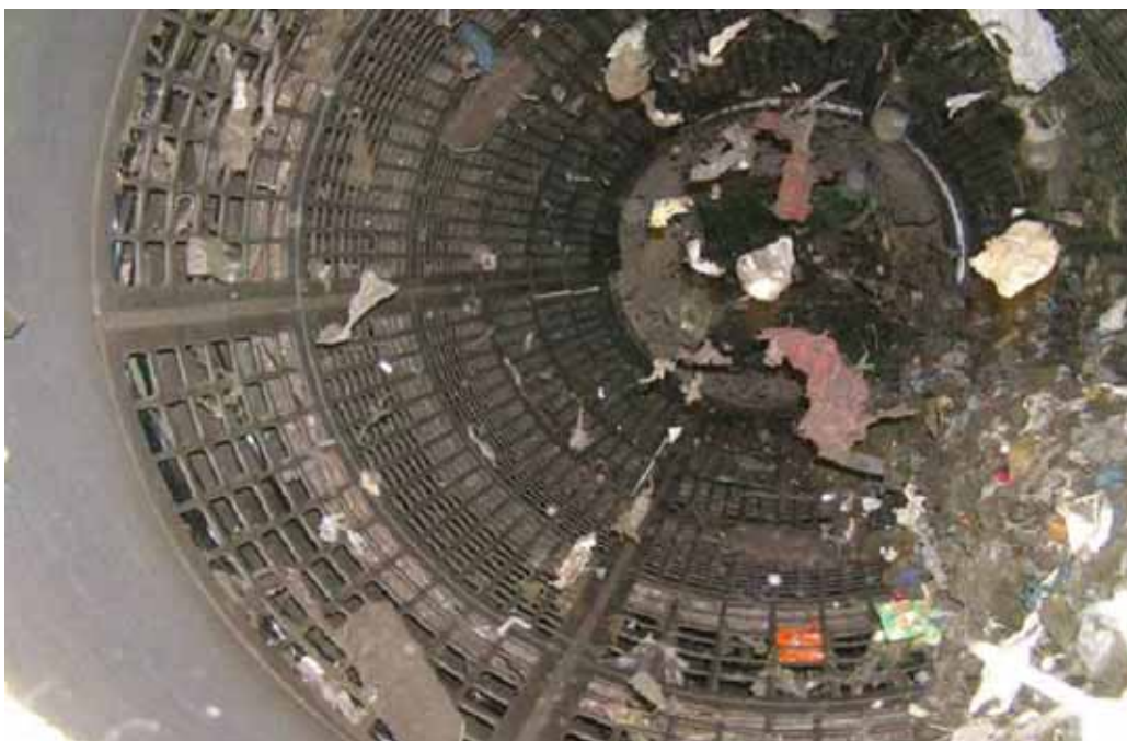
Figure 2: Waste separation using a trommel screen
